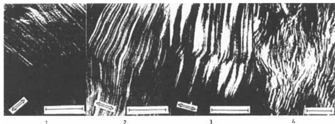
FIGURE 5 Electron micrographs of magnetically (and electrically) oriented films of polypeptides. 1. PBLG ( r = 470 ), 0.75 T; 2. an equimolar mixture of PBLG ( r = 470 ) and PBDG ( r = 530 ), 2.5 T; 3. PBLG ( r = 1,460 ), 180 V/cm; 4. same as in 2, no field. Cast and dried from methylene bromide solutions except 3 (methylene chloride solution). Bar, 5 \mu\text{m} ; the arrows indicate the direction of external field.
