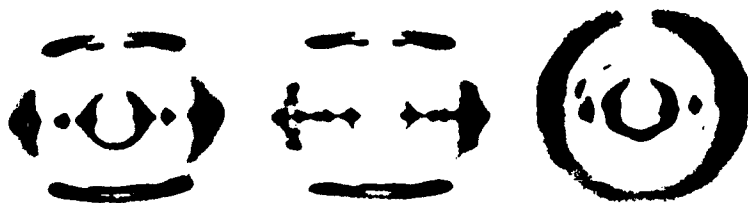
FIGURE 4 X-ray diffraction photographs of a magnetically oriented film of PBLG ( r = 650 ). Cast and dried from methylene bromide solution in the magnetic field of 0.96 T. Beam normal to film (left), parallel to surface of film (middle), both direction of magnetic field vertical, and along the direction of magnetic field, the polymer film being in a vertical plane (right). (By courtesy of Mr. S. Ejiri).
